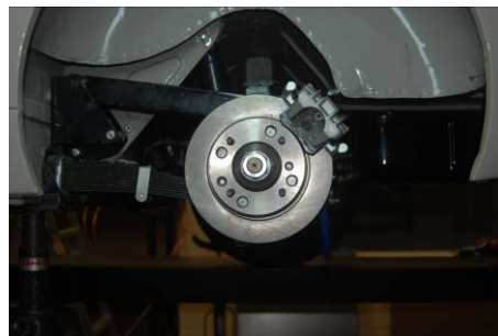
Fig 3 New caliper & disc fitted correctly on the axle
