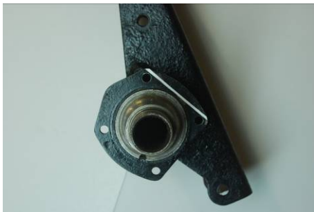
Fig 1 L/H brake mounting flange marked up ready for cutting
