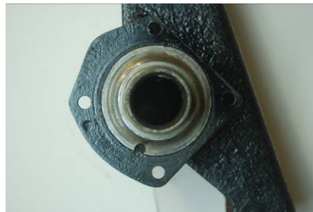
Fig 2 L/H brake mounting flange after the cut has been made
