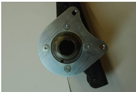
Fig 3 New caliper mounting plate bolted to the axle
